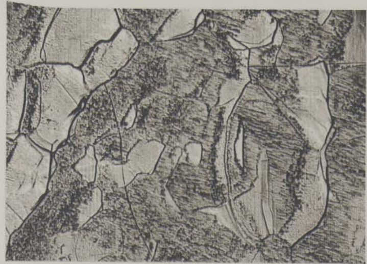
Bonding region on the copper surface
