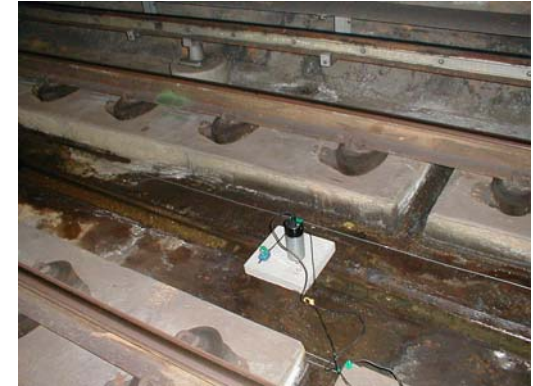
Typical receivers set-up Geophone & Accelerometer
