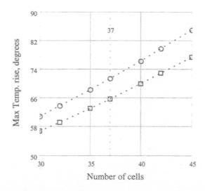
The distributions of the surface temperature rise after 130 ns in the 37-cell "nose" cone structure for the two currents and 120 MV/m gradient are shown next.
