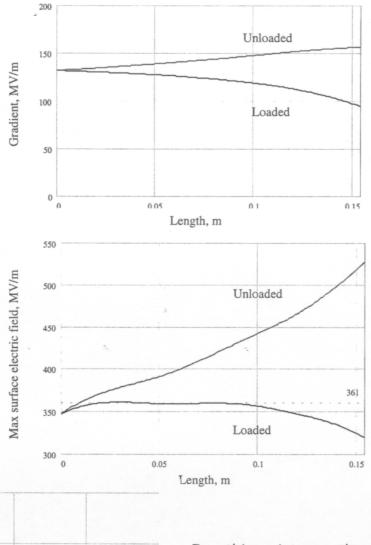
In this picture the maximal "unloaded" surface field of the "nose" cones structure as a function of the structure length is shown. Circles are the full current, boxes - 75% current.
