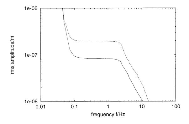
Longitudinal motion of the two tunnel ends at 34 m distance (velocity signals):
