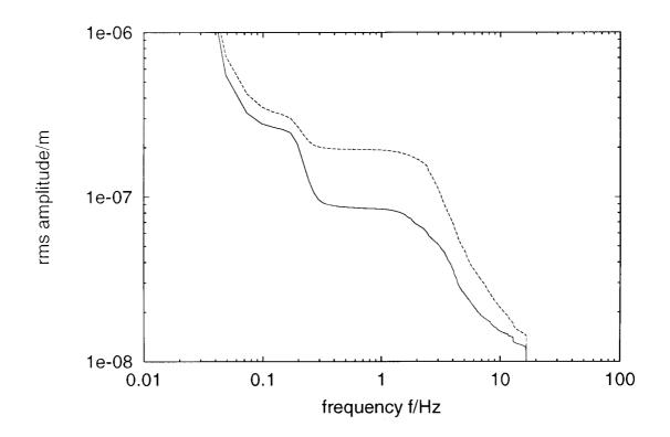
rms value of the difference signal  $x_1(t) - x_2(t)$  of the vertical motion of the two tunnel ends, distance 34 m, in the frequency range above  $f_0$ , given as a function of  $f_0$ :
