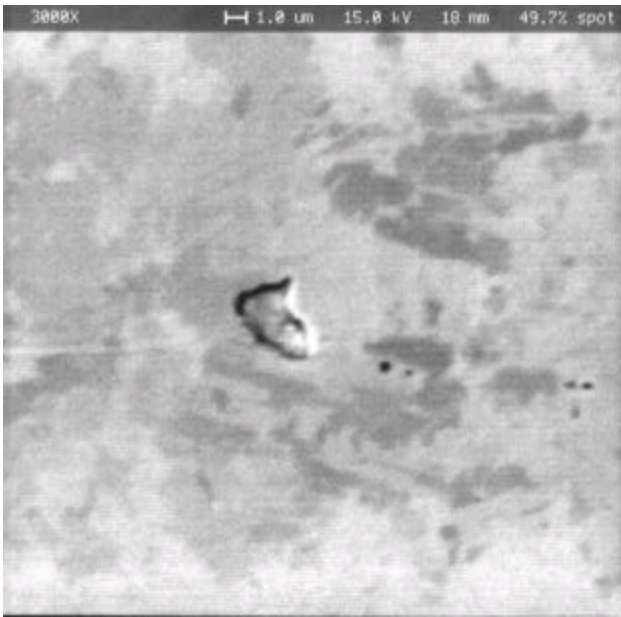
Figure 2. Missing copper grain and inclusions. Mottling is probably due to traces of cutting fluid on the surface.
