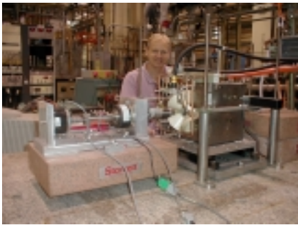
Zack Wolf, head of SLAC's Magnetic Measurement Group, with the NLC Prototype electromagnetic linac quadrupole in the SLAC rotating coil measurement set-up.
