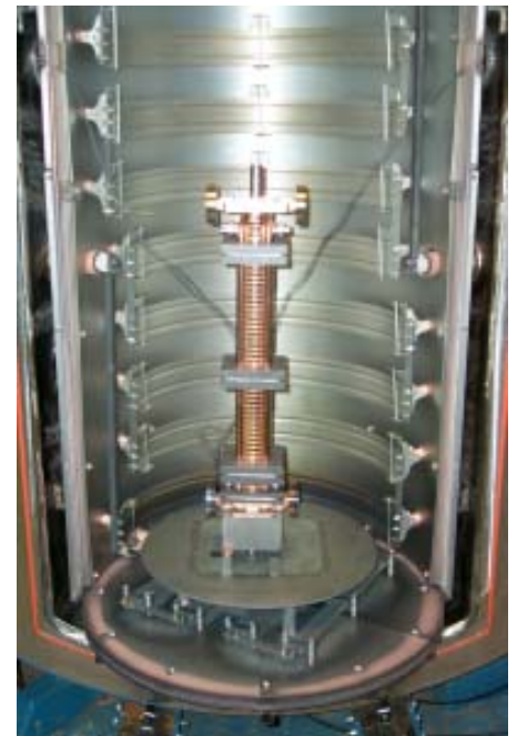
Figure 2: Brazing FXC-003 in our large vacuum furnace at IB4.
