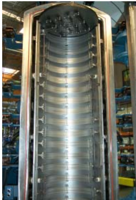
Figure 1: New hot zone installed in our large vacuum furnace at IB4.
