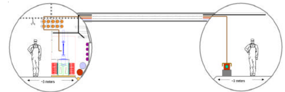
Figure 1-Schematic cross section of the NLC Support and the Beam Tunnels
