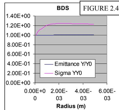
transverse beam size, we use a boundary radius of 400  $\mu\text{m}$  in the simulations; larger radii have little effect on either emittance or spot size (see Figure 2.4).
