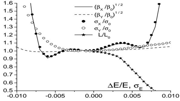
Figure 4: IP bandwidth of the traditional NLC Final Focus. Normalized betatron functions and normalized luminosity equivalent beam size (determined by tracking) versus energy offset  $\Delta E/E$ , and normalized luminosity versus rms energy spread  $\sigma_E$ .
