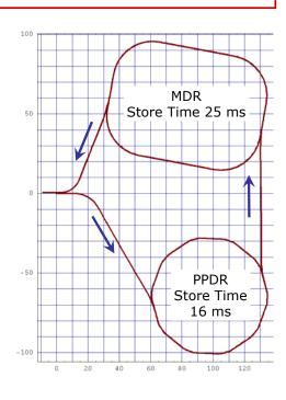
Top: Possible configuration for positron damping rings.
