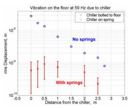
Vibration on the floor vs distance. For chiller on springs, its vibration effects are indistinguishable on the floor.
