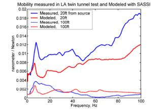
Mobility (response / driving force) measured in LA metro twin tunnel test and modeled with 3D code SASSI.
