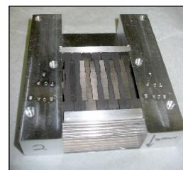
Radiation Damage Tests of Candidate Target Materials BNL
