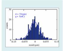
Histogram of the difference between the reading of BPM #2 and the line between BPMs 1 and 3
