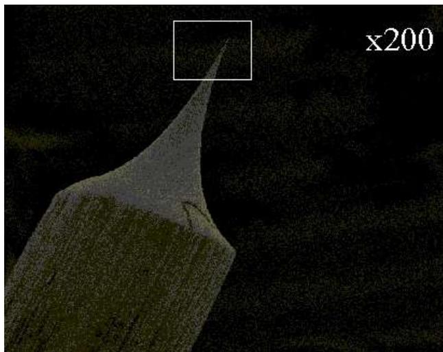
**Field emission:** Tungsten tips with radius  $\sim 10$  nm generate 100 MV/cm fields, enough to repel an ion from the surface. Ion release is well known, need to demonstrate operation in liquid xenon and ion trap.
