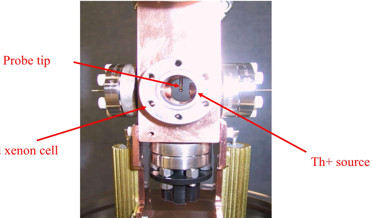
Probe collects Th<sup>+</sup> in liquid xenon,
